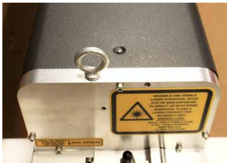
Figure 3-11. Eyebolts Installed in Laser System
