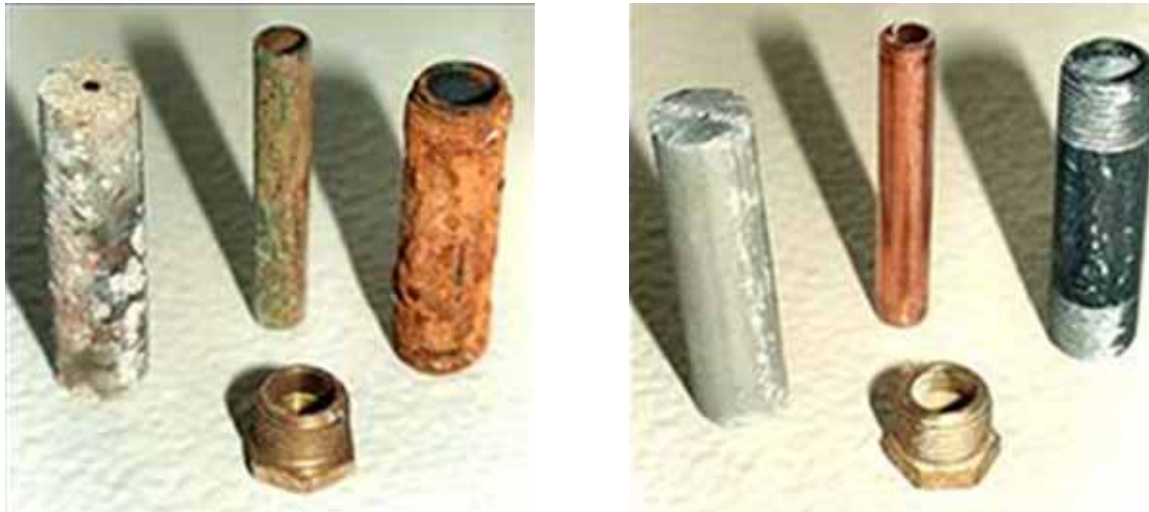
Untreated Water Circuit
